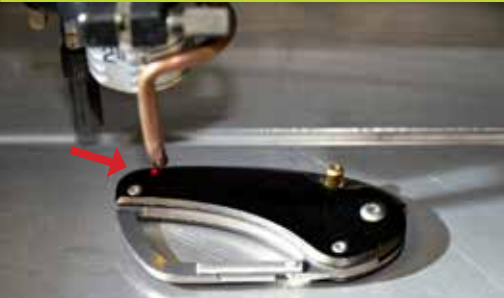
Acquisition of the shape to be engraved using the Point & Shoot red light pointer
