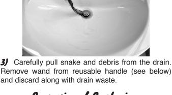
Removing / Replacing the Disposable Hair Clog Wand
