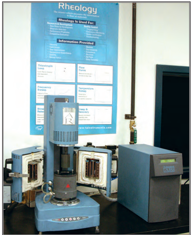
The Controlled-Stress Rheometer enables detailed characterization of a material's visco-elastic properties. This lets us predict the behavior of a material in a finished coating in more than ten ways (such as wettability, sag, stability, elongation, etc.).
