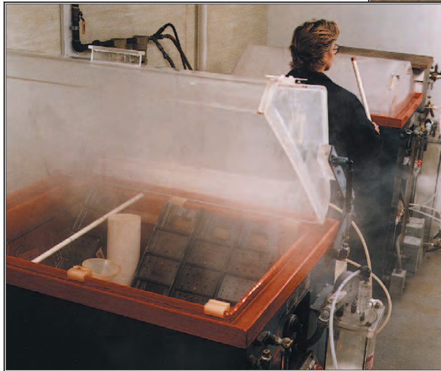
The salt-fog cabinets provide an accelerated method of determining the corrosion resistance of coatings exposed to the open air.
