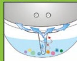
Rotation mixes air & water Dust, pollen & contaminants stay in water
