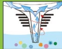
Rotation mixes air & water Dust, pollen & contaminants stay in water
