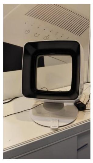
The oscillating windamp Air Fan (AF1010) has 8 speed settings, 8 timer settings from 1 to 8 hours and can be manually tiled 30 degrees.
