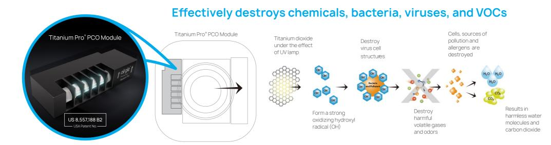
1) The Titanium Pro® module creates hydroxyl radicals by exposing titanium oxide (TiO<sub>2</sub>) to ultraviolet light. Hydroxyl radicals are naturally occurring molecules in the atmosphere. In fact, they are often referred to as the "detergent of the troposphere" because hydroxyl radicals destroy many airborne pollutants by breaking apart the molecules of the pollutant.
